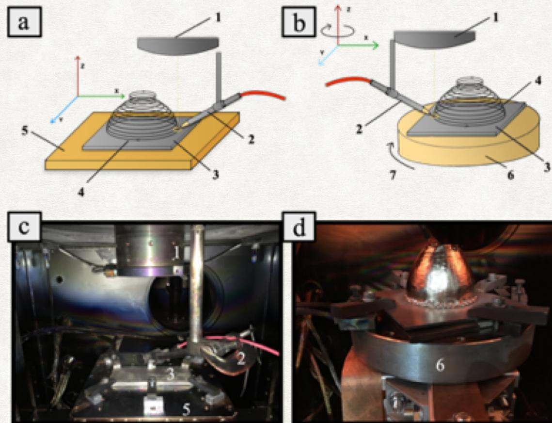
The schemes of obtaining the samples and photos of vacuum chamber with a standard 3-axis water-cooled table (a, c) and rotating uncooled table (b, d). 1 – Electron beam gun, 2 – Wire feeder, 3 – Substrate, 4 – Spiral trajectory of the sample formation, 5 – Three-axis water-cooled table, 6 – Uncooled rotating table, 7 – Direction of rotation.
