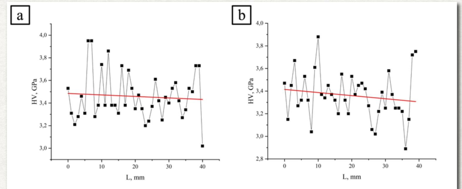
Microhardness of the sample, manufactured on the 4-axis table (mode II) in different sections
