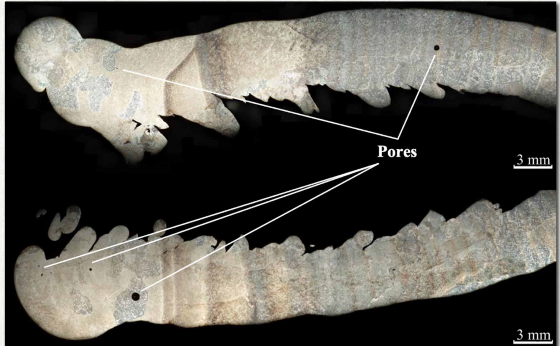
Macrostructure of the sample at different wall sections
