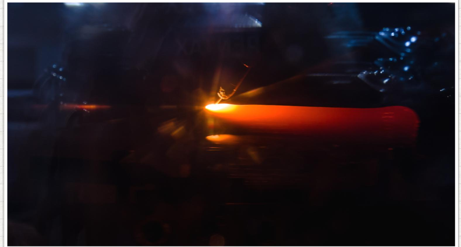
Electron-beam additive manufacturing (EBAM, EBF<sup>3</sup>) is a technology based on wire feeding into a molten bath. The process occurs in a vacuum and the molten bath is formed by an electron beam.
