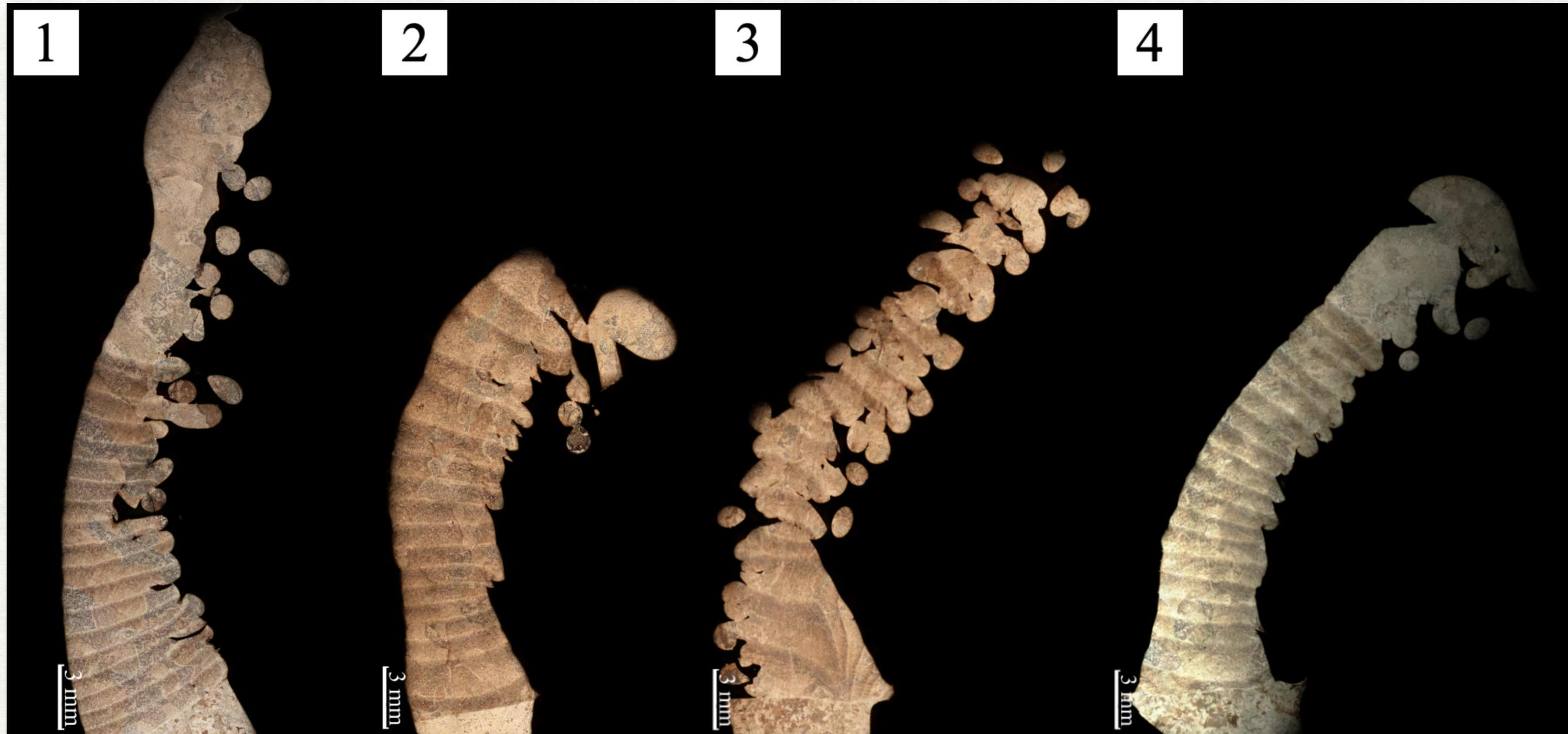
Macrostructure of the sample in areas affected by the wire feed geometry
