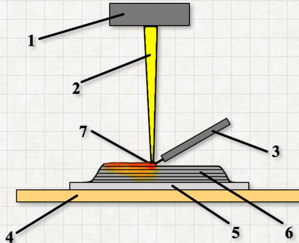
1 – Electron-beam gun, 2 – electron beam, 3 – wire feeder, 4 – cooled table, 5 – substrate, 6 – printed sample, 7 – molten bath
