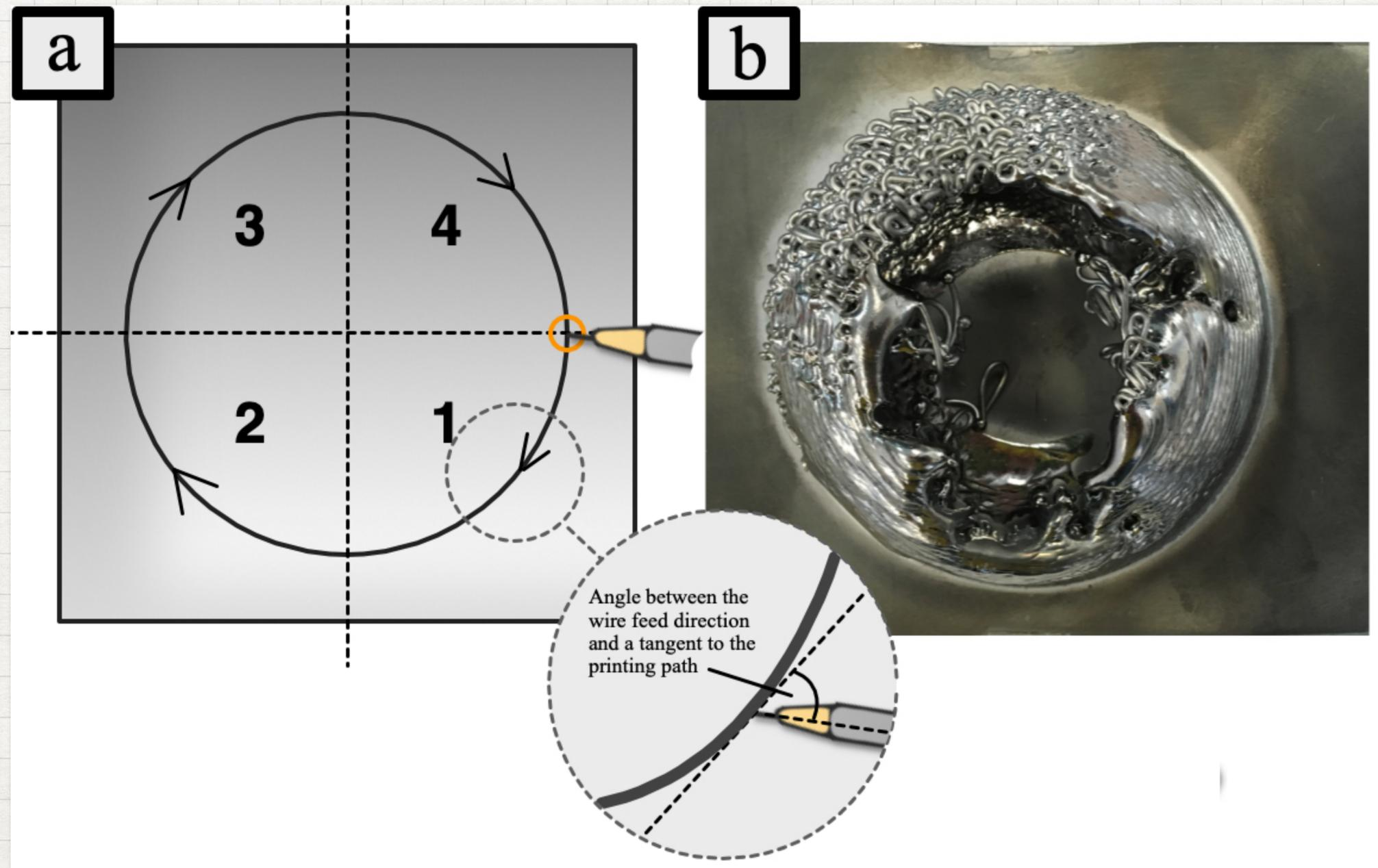
The geometry affected zones on samples manufactured with the use of the standard 3-axis table:
