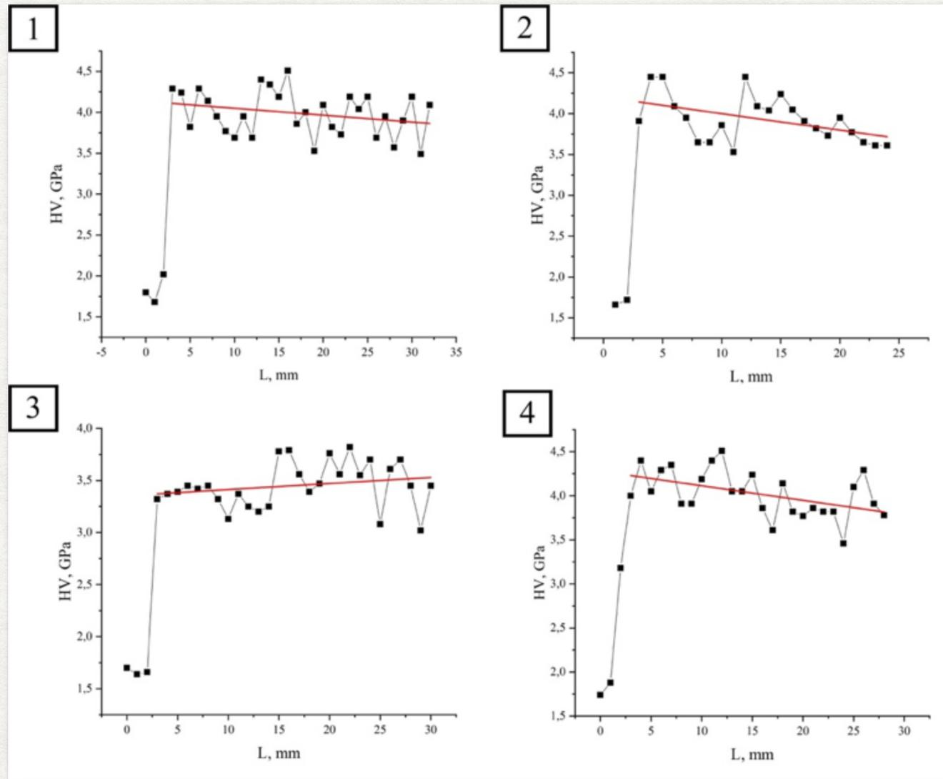
Microhardness of the sample, manufactured on the 3-axis table (mode I) in geometry affected zones
