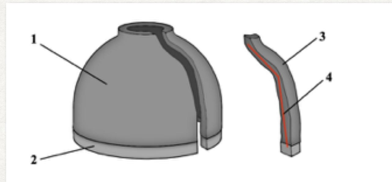
The scheme of cutting the templates and measuring microhardness.
