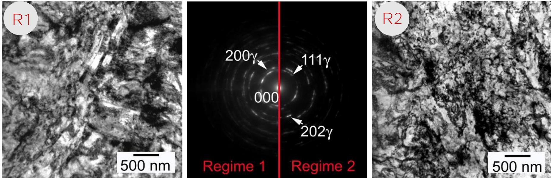
Two types of grain-subgrained structures in steel
