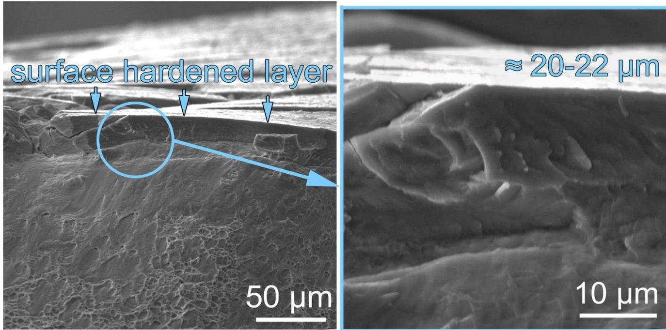
IPT facilitates a formation of composition hardened surface layer  $\approx 20-22 \mu\text{m}$  in thickness
