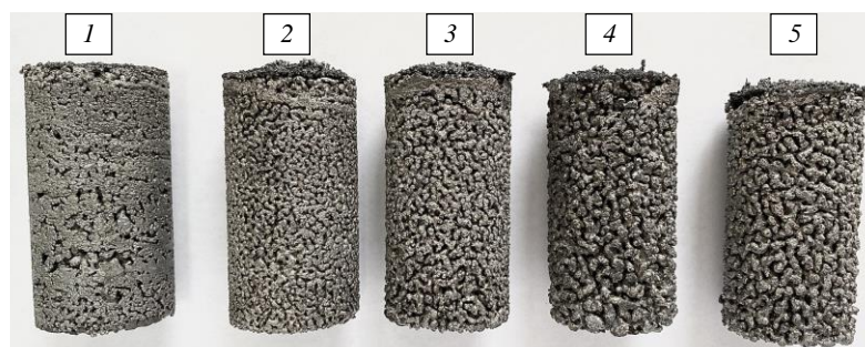
Figure 1. Images of synthesized alloys depending of the thickness of a barrier layer h made from the office paper. Part 1 – without barrier layer. Part 2 – h = 108 micron, Part 3 – h = 216 micron, Part 4 – h = 324 micron, Part 5 – h = 432 micron.
